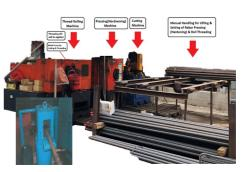
Good quality threads should be required by frequent change of tooling & strict inspection checking (QITP) which included go & no go gauge for thread length & pitch gauge for thread accuracy
