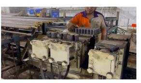
On-site Rebar Coupler Fabrication by ONE-GO PROCESS
